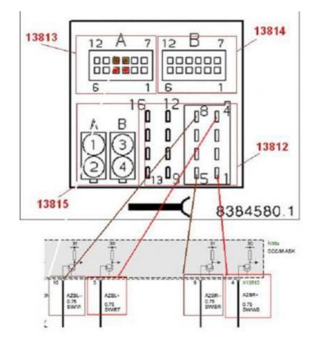
What you need to do is remove pins 3, 4, 9 and 10 from the 13813 block. Leave the pins in 13812 in their socket! Now using for example tap connectors you connect the loose wires that were in block 13813 to the wires in socket 13812 in the following order:
