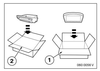
Place the removed 6.5" on-board monitor in the packaging (1) of on-board monitor **B**.
