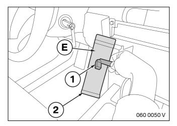
Cut apart the protective strip **E** at right angles to the adhesive strips in the middle.
