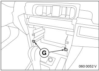
Attach speed nuts **G** to the centre console module holder.
