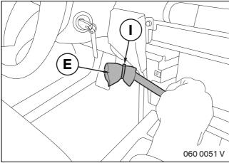
Also secure protective strip **E** using cable tie **I**.
