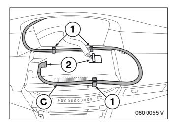
Secure LVDS cable **C** in a broad arc in the holders (1) of 8.8" on-board monitor B.
