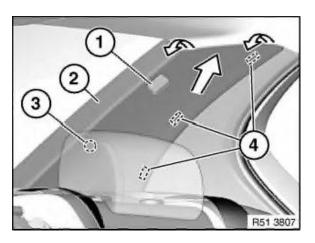
Lever out airbag emblem (1) and release screw underneath.
