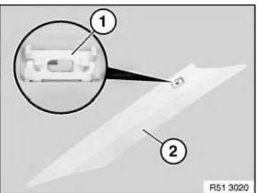
Installation: Retainer (1) on trim (2) must not be damaged or missing.
