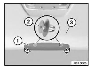
Unclip cover for auxiliary brake light (1) at points (2) and feed out sideways in direction of arrow.
