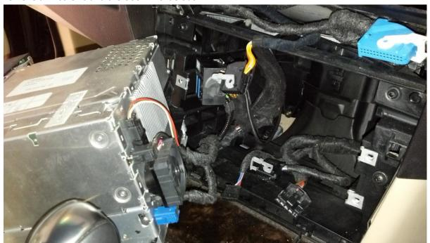
You need to remove all the plugs from the CCC, Each is different or colour coded. Place the CCC to one side.
