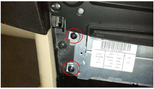
Remove all 4 screws and the CCC will slide out.
