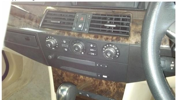
As the trim comes away there is the Hazards/Lock/Unlock button to unplug, this just pulls off. I find it easier to remove the button from the trim. The Air vents are attached to the trim piece, so no need to worry about them.
