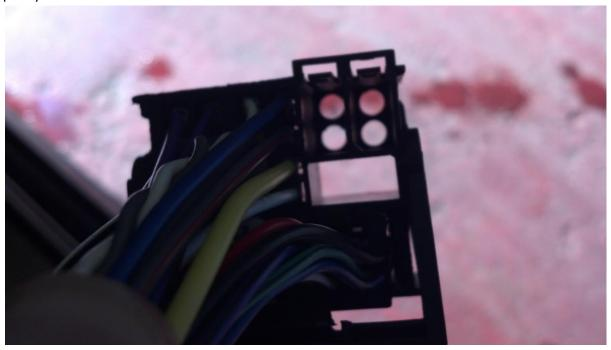
6. With that done you need to attach the aerials harness to the CCC. The aerial is the Black socket on the CCC (the blue is the GPS), Also connect the car's harness to the supplied one.
