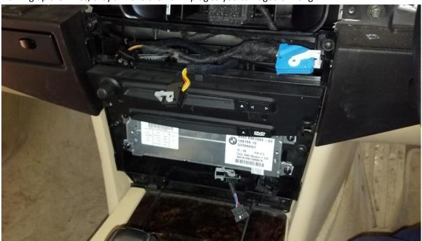
4. Next step is the Radio/CCC, It's held in by 4 screws.
