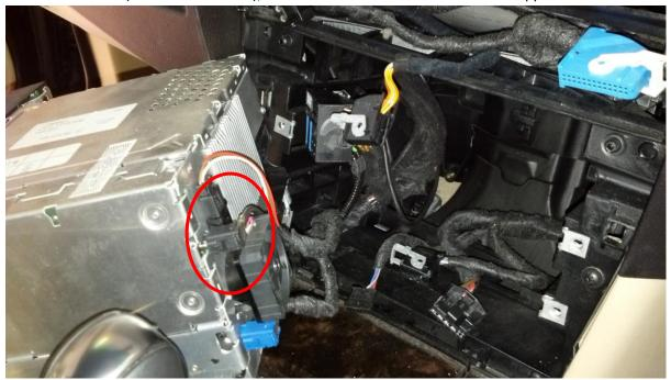
7. Mounting the DAB unit. I've put mine under the steering wheel and threaded the wire to it from the CCC. There is no space for it behind the CCC so it's either under the wheel or behind the glove box. Whichever side you choose push the 2 ends of the aerial through (the
