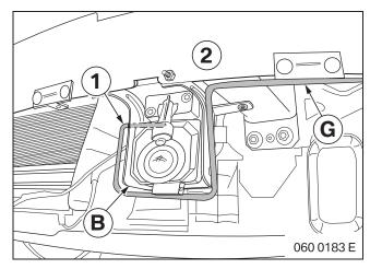
Install high pressure line **G** according to **TIS 61 67 010**. Route the branch (1) of line G to camera B beneath the aluminium mounting (2).
