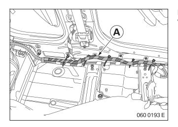
Route cable kit  $\boldsymbol{\mathsf{A}}$  along the vehicle wiring harness on the vehicle floor.
