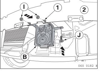
Insert the stud (1) of assembly camera **B** into the existing bore holes of the aluminium mounting (2) from the rear. Mount camera **B** on the aluminium mounting (2) with nuts **I** and bolt J.
