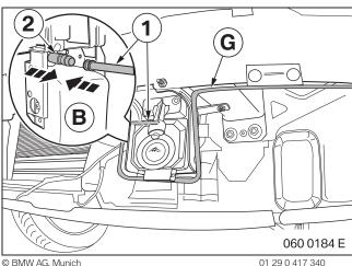
Connect the branch (1) of line G to the injection nozzle (2) of camera **B** from the rear.
