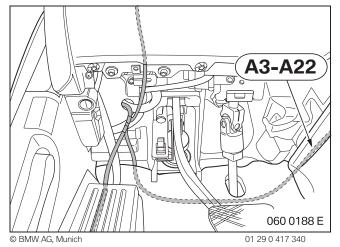
Route connecting points **A3** to **A22** behind the heater to the fuse carrier in the glove box.
