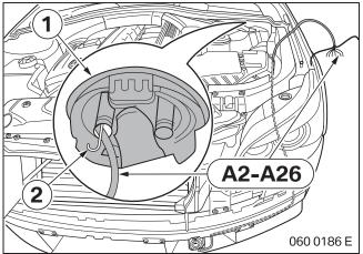
Pull connecting points **A2** to **A26** into the car interior through the rubber grommet (1).
