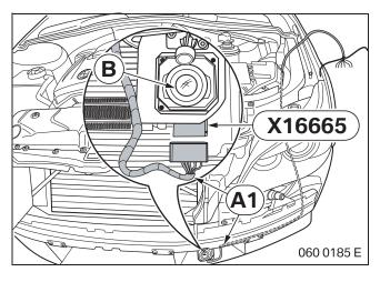
Route connecting point **A1** to camera **B** along the vehicle wiring harness.
