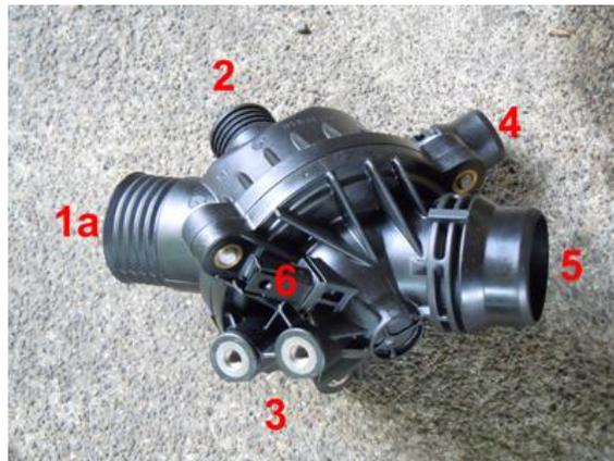
The thermostat is held in places with two 10mm bolts that are screwed in through mounts on the water pump. In pictures 1297a and 1301a they are both marked with #3.
