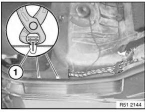
Lever out clips (1) with pliers (head of pliers surface-ground).
