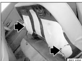
Unclip rear seat on left/right towards top. Lift out seat.
