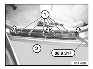
Unclip clips (1) for finishing strip (2) with special tool  $00\ 9\ 317$ . Remove finishing strip (2).
