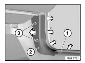
Release door mucket (1) in area of footwell side trim panel on Apillar on right (2).
