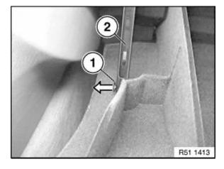
Unclip pin (1) from shock absorber (2).
