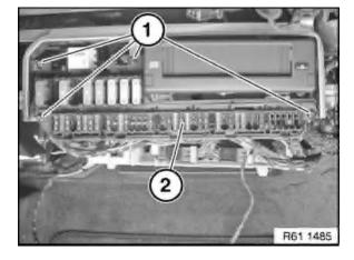
Release screws (1) and remove distribution box (2).
