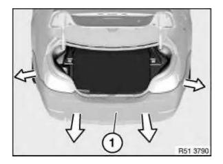
Unclip bumper trim (1) to side panel (1) on left/right outwards. Remove bumper trim (1) in direction of arrow towards rear. With optional extra PDC:
