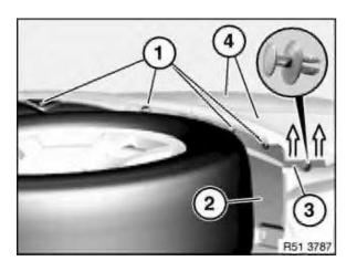
Release screws (1) from wheel arch cover (2) on left/right. Release expansion rivet on left/right.
