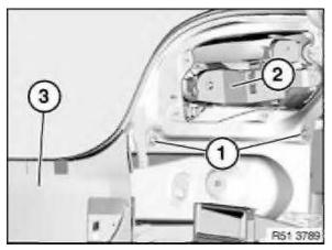
Release screws (1) with sealing washers on left/right.
