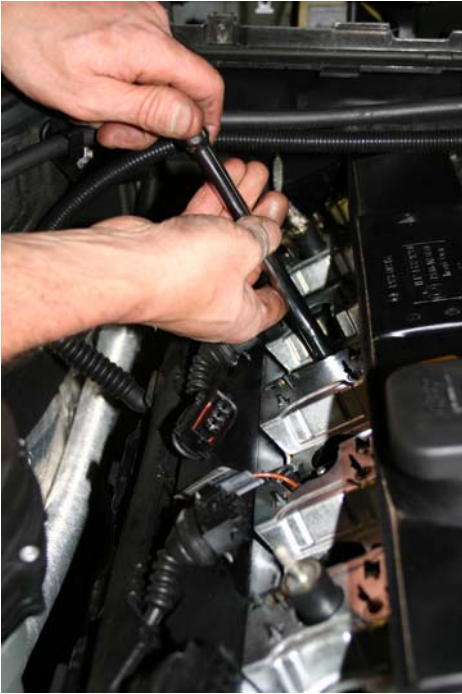
Replacing spark plugs in an M54 engine.
