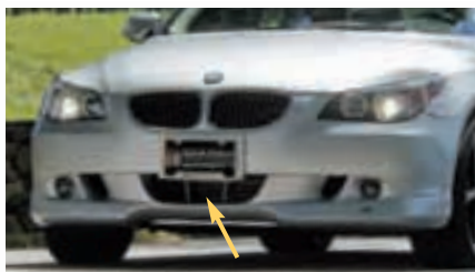
Inside lower center grill opening: 3 series 06 on, 5 series 04 on, 6 series 03 on, 7 series 02 on.
