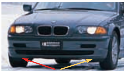
Splash panel under bumper: driver's side (yellow arrow) on 3 series 99 thru 05; passenger's side (red arrow) on 5 series 89 thru 03, 7 series 88 thru 01.
