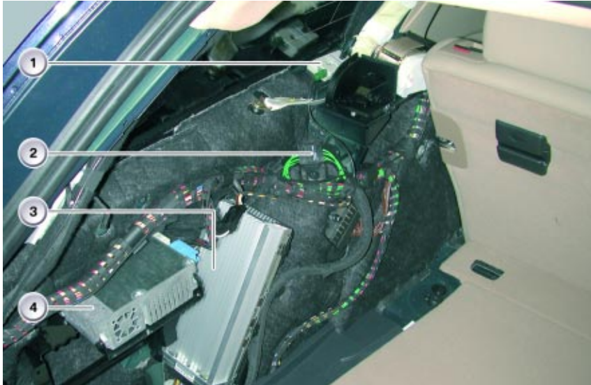
Control Units in Luggage Compartment, Left
