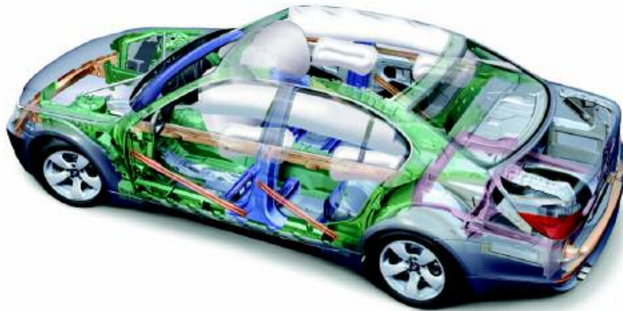
BMW Safety Concept with Safety Passenger Cell and Airbag Systems (E60)
