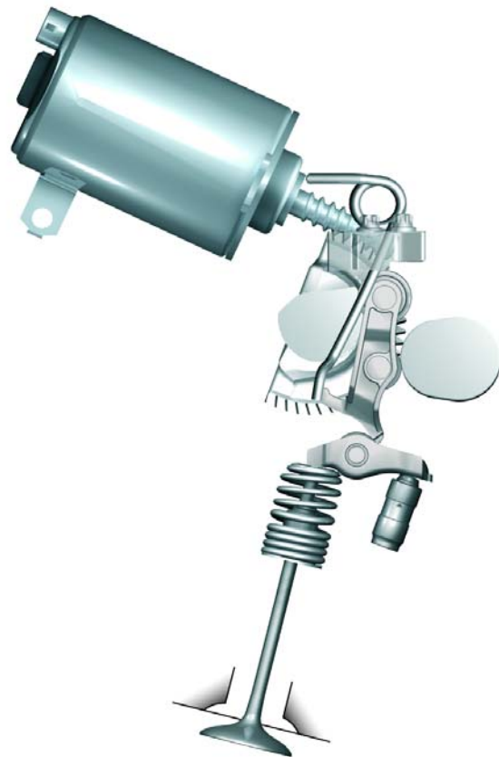
Valvetronic II at maximum valve lift
