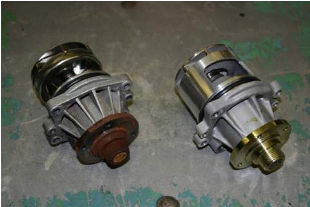
Problematic OE/OEM water pump (l), compared with EMP Stewart High Performance Water Pump. Yes, the pump on the left has a metallic Impeller – that doesn’t make any difference in longevity. Both the plastic and metallic impeller OE/OEM pumps fail prematurely, just in different ways.
