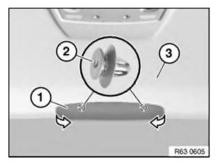
Unclip cover for auxiliary brake light (1) at points (2) and feed out sideways in direction of arrow.
