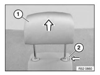
Move head restraint (1) upwards to maximum extent. Press lock (2) and pull out head restraint.
