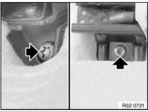
Release front screws on left and right seat rails. Tightening torques 52 10 1AZ
