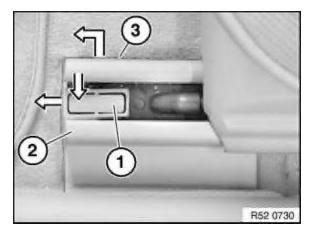
Press rocker switch (1) on front left seat rail cover and unlock. Gently slide cover (2) towards front.
