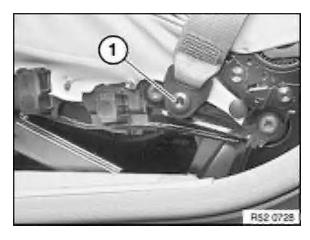
Release screw (1) for belt mounting. Tightening torque 72 11 11AZ.
