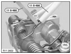
Attach special tool 11 9 490 to second end of torsion spring. Support end of torsion spring protected with special tool 11 9 490 on inlet camshaft.
