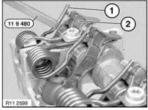
Hold torsion spring (1) with special tool 11 9 480 . Install intermediate lever (2) from above. Insert end of torsion spring (1) into guide on intermediate lever (2).
