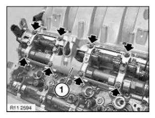
Release 8 nuts of bearing bracket (1) from outside to inside.
