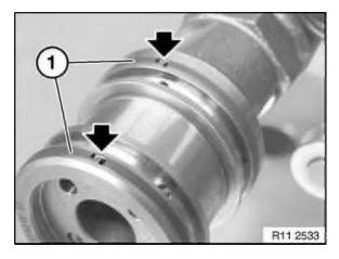
Ends of compression rings (1) point upwards.
