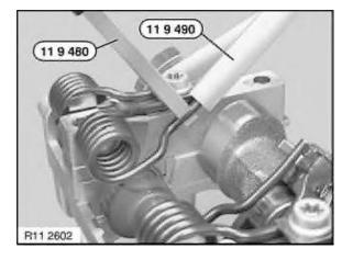
Raise torsion spring (1) with special tool 11 9 480 . Detach special tool 11 9 490 .
