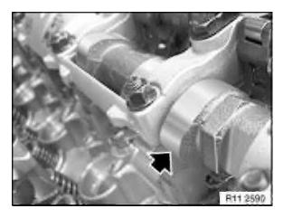
Rotate inlet camshaft in direction of rotation until cam on 1st cylinder is positioned horizontally as shown in illustration.
