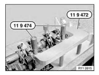
Insert special tool 11 9 474 and initially tighten without play.
