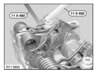
Attach special tool 11 9 490 to end of torsion spring. Support end of torsion spring protected with special tool 11 9 490 on inlet camshaft.
