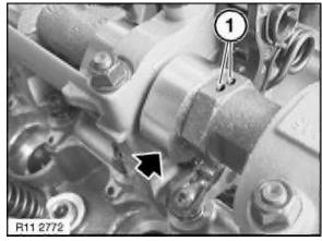
Rotate inlet camshaft at hexagon head against direction of rotation until cam on 1st cylinder points points downwards at an angle as shown in illustration.
