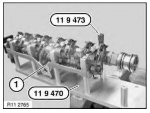
Place bearing bracket (1) with inlet camshaft and eccentric shaft as illustrated on special tool 11 9 470 .
