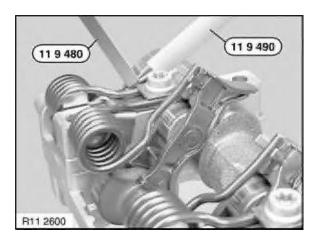
Raise second end of torsion spring with special tool  $11\ 9\ 480$  . Detach special tool  $11\ 9\ 490$  .
