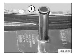
Replace sealing ring (1) on oil filter tube.
