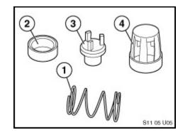
Engine Oil Pump Non-Return Valve Parts:
