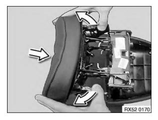
Bringing head restraint together - version without button (MFS): Pull spring catches apart and push head restraint together. Maintain position.
