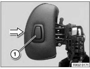
Bringing head restraint together - version with button (Basic): Press button (1) and push head restraint together.
