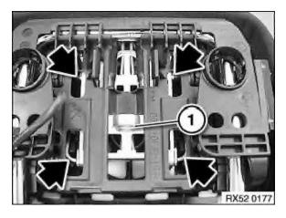
Checking head restraint lock:
