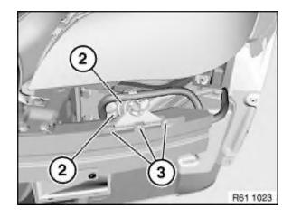
Unlock high-pressure line (1) and detach from high-pressure nozzle (2).
