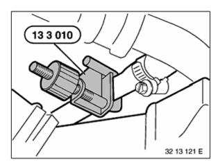
To prevent excessive escape of washer fluid, seal off end of high-pressure line with special tool  $13\ 3\ 010$  .
