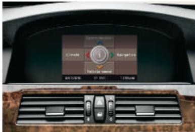
■ **Control Display** (6.5 inch, colour) for displaying functions that are accessed using the Controller (e.g. on-board computer or radio).
