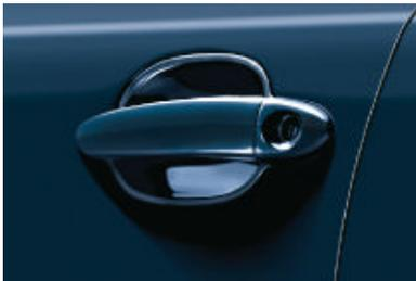
□ **Soft Close Automatic** system gently closes all four doors (kicks in for the last 6 mm of travel), using an electric motor.
