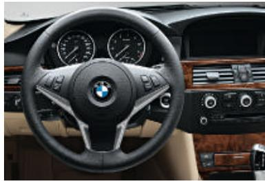
□ **Sports leather steering wheel**, very comfortable grip thanks to small diameter (379 mm), three spokes, with multifunction buttons; the integrated buttons can be used to operate the radio, CD drive and telephone (optional) while on the move. Two buttons are available for user-defined functions.
