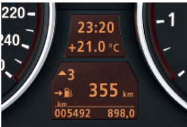
■ **Optimum Shift Indicator** shows when switching to another gear would be more fuel-efficient. The system recommends when to switch to a higher or lower gear, as appropriate for your driving style. For example, when accelerating, a signal is shown at the point where you could continue to accelerate in a higher gear while however saving fuel (for vehicles with 6-speed manual transmission).
