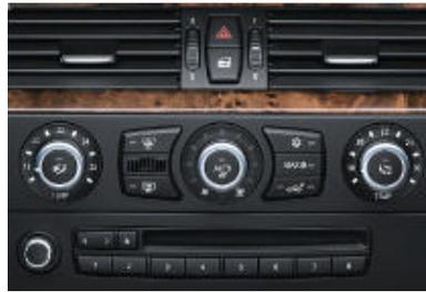
□ **Automatic air conditioning, extended** with AAR, solar sensor and fogging sensor, automatic temperature control and air distribution (separate for driver and passenger) also air volume control; status and settings shown on the Control Display. With adjustable armrest and air-conditioned storage tray in centre console (standard on 540i, 550i and 535d).
