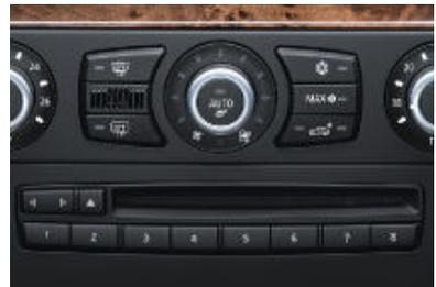
■ **Functional bookmarks:** The driver's and passenger's most frequently used navigational targets and telephone numbers or specific CD tracks can be individually stored on eight separate buttons and accessed with a click.
