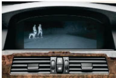
□ **BMW Night Vision** uses an infra-red camera to detect people and animals up to a distance of 300 metres. The camera images appear in the Control Display. This enables you to see obstacles that are still out of range of the headlights, so you can react in good time.
