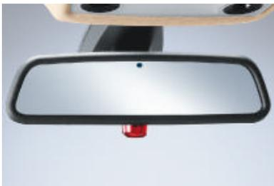
□ **Interior mirror with automatic anti-glare function**, large surface area; the glare from following vehicles is automatically reduced when the amount of incident light exceeds a defined limit.
