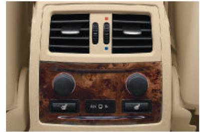
■ **Fresh-air outlets** at the rear. In conjunction with automatic air conditioning with extended features (shown here), these outlets provide temperature-controlled ventilation of the rear.
