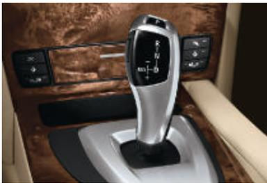
□ **6-speed automatic transmission** with Steptronic. The gearshift mechanism enables very fast, immaculate gear changes – for truly dynamic performance (standard on 535d).
