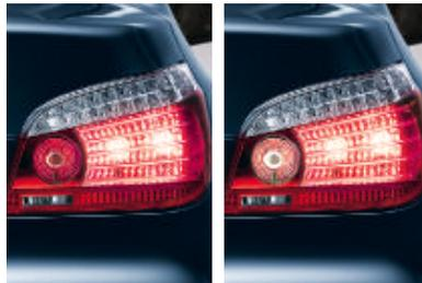
■ **Brake Force Display** helps vehicles travelling behind you to evaluate your braking more accurately: in the event of an emergency stop, the illuminated area of the brake lights is increased. So traffic travelling behind can tell in an instant the difference between a light tap on the brake pedal and a hard stop – for increased driving safety.
