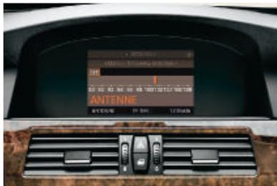
■ **Radio Business**, 4-channel amplifier, aerial diversity, scan function, CD drive with title scan and automatic CD insert/eject, six loudspeakers and MP3 decoder.
