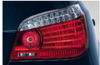
■ **Rear light** with LED indicators and five radial LED light conductors ensures optimum recognition even in poor visibility. Clear glass sets off this high-quality, modern lighting technology, making for an individual appearance.
