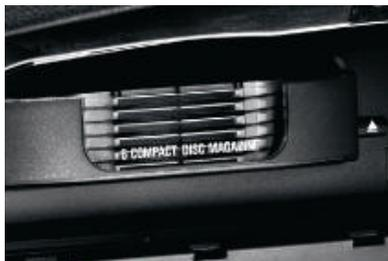
□ **CD changer**, for six CDs, integrated into the glove compartment.
