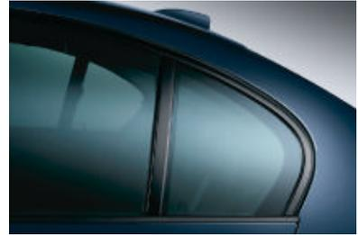
□ **Shadow Line** comprises front and rear side-window frames and window recess finishers in Black, matt.
