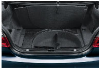
□ **Compartments** underneath the level luggage compartment floor offer additional storage space (in conjunction with runflat tyres).
