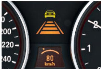
□ **Active Cruise Control with Stop & Go function.** Driving assistance system for increased comfort and active safety in particular for driving in slow-moving traffic. Combines Cruise Control with active safe distance control to a stand-still in bumper-to-bumper driving, with automatic restart in typical "Stop and Go" situations.
