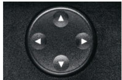
□ **Lumbar support** for driver and front passenger seat, in height and depth electrically adjustable, for ergonomically perfect seat position and support of the back muscles.
