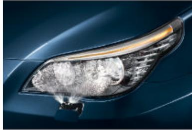
□ **Headlight washing system** ensures optimum headlight brightness in all kinds of weather. When the lights are on, the headlights are automatically cleaned in parallel with the windscreen (only in combination with Xenon lights\*).
