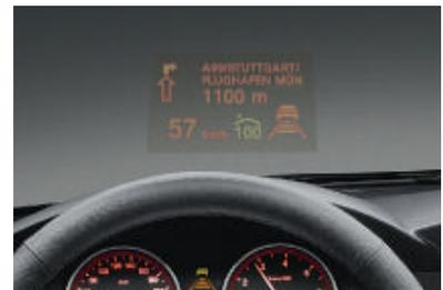
□ **Head-up Display** projects relevant data, such as the current speed, directly into the driver's field of vision. Other display data include direction arrows from the navigation system\*, Active Cruise Control functions with Stop&Go function, Lane Departure Warning System and Check/Control data.
