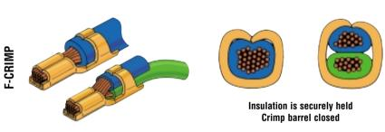
For double wire applications with different size wires always place wire with smallest outer diameter in the bottom
