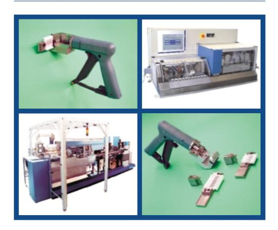
Tyco Electronics is the worldwide leader in the field of interconnection devices utilizing Insulation Displacement technique (IDC). A comprehensive range of application equipment is available, from hand tooling up to fully-automatic equipment.
