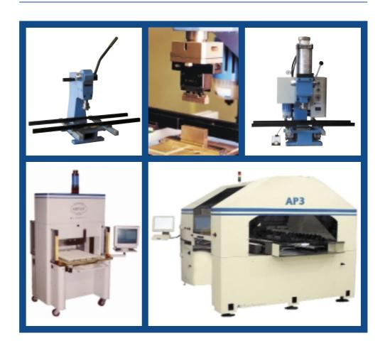
Tyco Electronics is one of the leading manufacturers and suppliers of ACTION-PIN connector seating equipment varying from hand operated arbor presses, C-frame type pneumatic presses to fully-automatic servo electric PC controlled machines and accessories.
