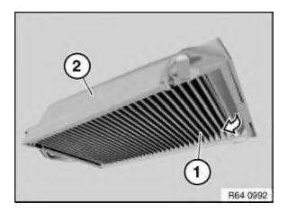
Lever microfilter for interior ventilation (1) in direction of arrow out of microfilter air duct (2) and remove.
