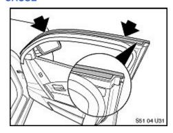
Movement between the flocking material (felt-like material indicated by the arrows) on the upper door seal and the surrounding roof panel may produce squeaking or creaking noises.
