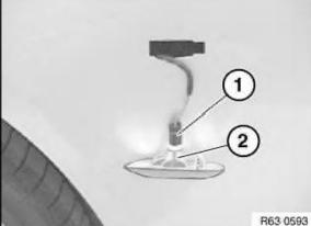
Unfasten plug connection (1) and disconnect. Remove front auxiliary turn signal lamp (2).
