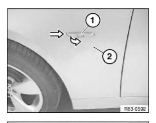
Slide from auxiliary turn signal lamp (1) towards rear and fold in direction of arrow out of front side wall (2).
