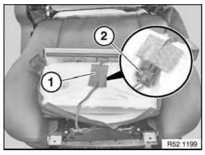
For seat heating optional extra only: Carefully detach felt (1) from thigh support. Unfasten plug connection (2) and disconnect.
