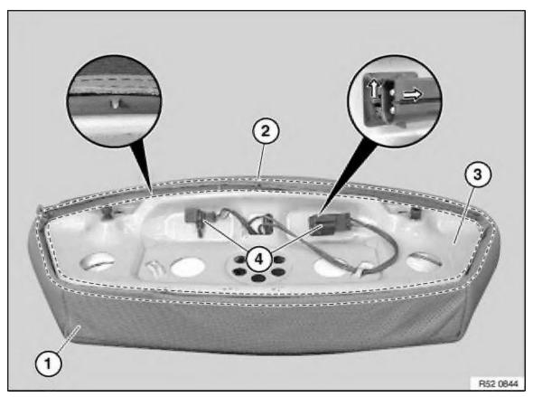
The work operations here are shown on the version with air conditioning and seat heating. Feed out seat cover (1) in area (2).
