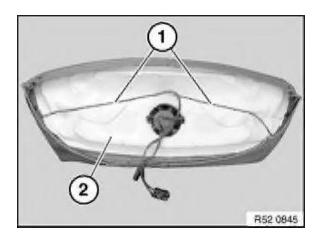
Version with seat heating or air conditioning: Feed out cable (1) and remove padding (2).
