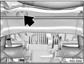
If necessary, unclip scavenging air line and screw off bracket. Release nut and pull out screw towards rear.
