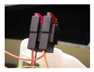
14. Relock the connector and reinstall the relay. Mount the retrofit harness fuse holder and 10 Amp fuse holder in the original factory location.
