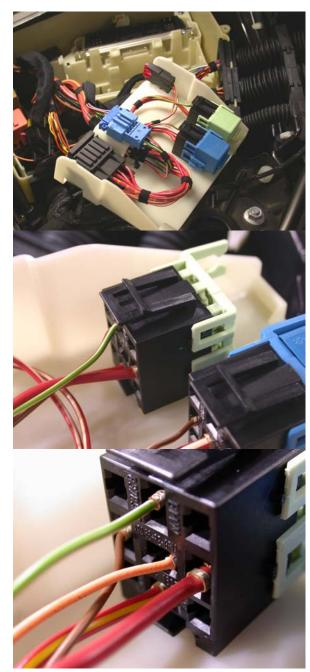
13. Remove the adjacent 10 Amp fuse holder and attach retrofit harness fuse holder to one another.
