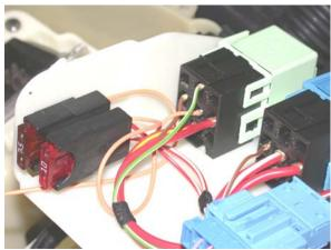
15. Reinstall all components in E-Box to their proper locations. Replace the Oil Condition Sensor, reconnect the vehicle battery and clear fault code memory using the DIS Plus or GT1 Diagnostic device.
