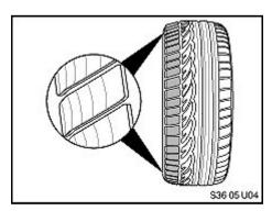
Check all four tires for proper inflation pressure and tread wear each time a customer comes into your center.
