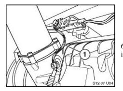
6. Position the ground cable (1) as shown on the illustration.
