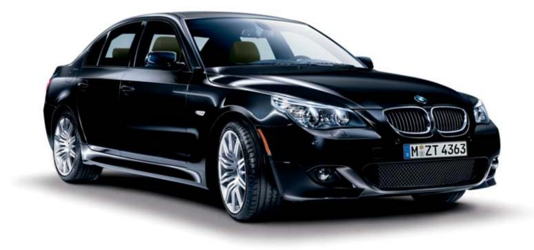
**Aerodynamic package's** front air dam and bumper underscore the purposeful look of the 550i, while providing a visual clue to the power of the 4.8-liter V-8 that resides under the hood.
