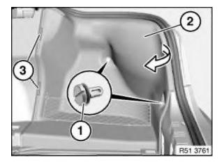
Open rotary clips (1) and remove.
