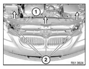
Unclip strip (1) in direction of arrow and release screws (2) underneath.
