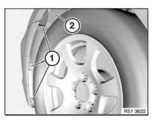
Release screws (1) on wheel arch trim (2) on left/right.
