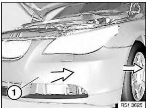
Press bumper trim (1) against direction of travel and release from holders in direction of arrow.
