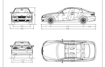
All dimensions in millimetres. Luggage compartment capacity (VDA method): 440 litres: 335i: 430 litres.
