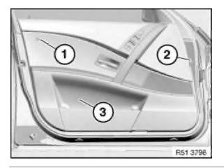
Lever out airbag emblem (1) with special tool 00 9 317 and release screw underneath.
