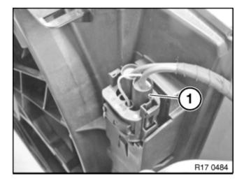
Unlock connector (1) and pull off.
