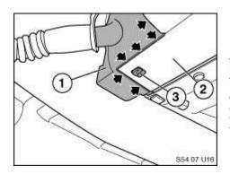
b. If any water seepage is observed, apply sealant to the seam where the drain pocket (1) meets the cassette (2). The retaining tab (3) must also be sealed. Wurth Euroseal Gel or a comparable silicone sealant may be used for this procedure.
