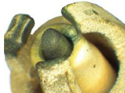
Spark plug showing abnormal wear pattern - look for possible fuel spray diversion
