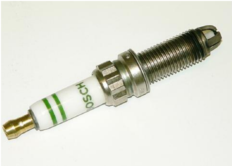
Spark plug showing abnormal wear pattern - look for possible fuel spray diversion
