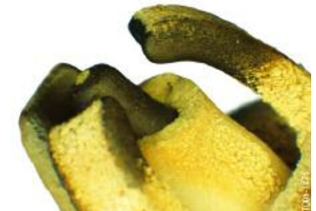
Spark plug showing abnormal wear pattern - look for possible fuel spray diversion
