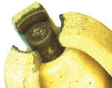
Spark plug showing abnormal wear pattern - look for possible fuel spray diversion
