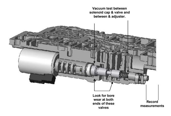
The solenoid OD, its end cap and the adjuster must seal oil circuits.
