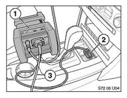
7. Disconnect the OPPS/OPS from the OBD connector and plug special repair cable 52 1 010 (3) into both OPPS/OPS (1) and into power supply (2).
