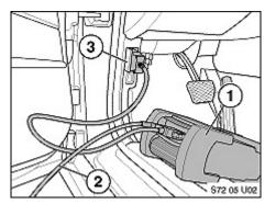
13. Reconnect the OPPS/OPS (1) to the vehicle using the regular diagnostic (OBD) connector (2).
