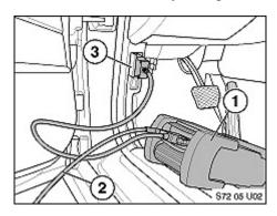
2. Connect OPPS/OPS (1) to the vehicle OBD connector (3) and to the network (or directly to the GT1) (1).
