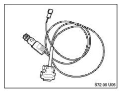
For E60/E65/E66 with Sport Seats New or Comfort Seats and E90 only, use special repair cable 52 1 010 to recode the OC3 seat occupancy mat (do not replace parts):
