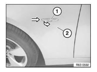
Slide from auxiliary turn signal lamp (1) towards rear and fold in direction of arrow out of front side wall (2).
