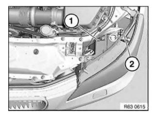
Adjust headlights at adjusting screws (1) and (2). A definite allocation of adjusting screws is not possible.
