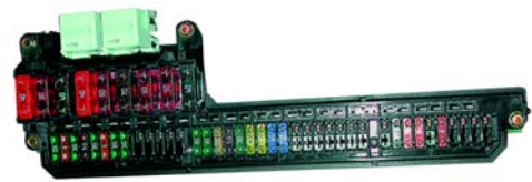
Front Power Distribution Box
