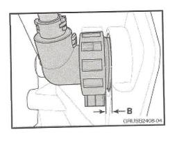
After installation, the correct distance between the transmission harness connector and the housing surface (B) should not exceed 3 mm.
