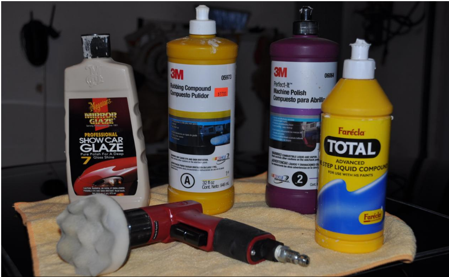
Compound, polishing compound, polish and glaze. Also you need 2000-3000 grit wet paper
