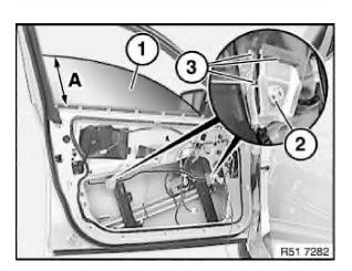
Door window glass (1) must be opened to dimension (A). A= approx. 205 mm Release screws (2). *Installation:* Rubber (3) must be correctly fitted. Tightening torque 51 32 2AZ .
