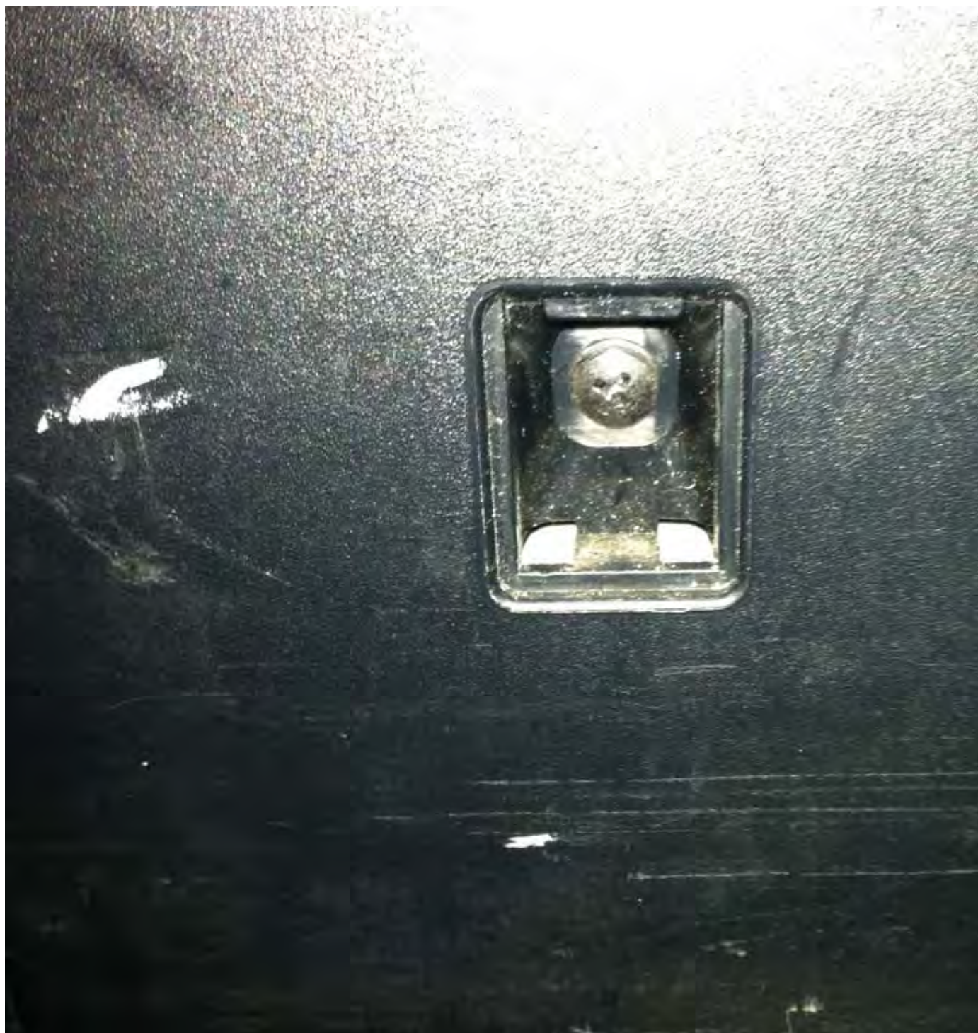
The other screw is located near driver side cargo hook anchor.
